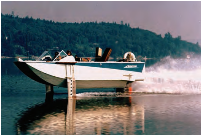
Left: Boeing's "LITTLE SQUIRT" was a 20-foot long hydrofoil research craft built in 1962. It tested automatic control systems and was the first hydrofoil to demonstrate the use of water-jet propulsion. Photo courtesy The Boeing Company.
