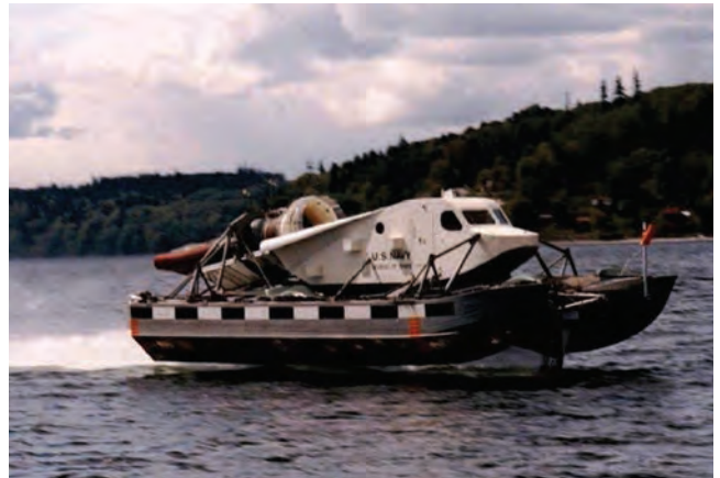
Left: Boeing's "LITTLE SQUIRT" was a 20-foot long hydrofoil research craft built in 1962. It tested automatic control systems and was the first hydrofoil to demonstrate the use of water-jet propulsion. Photo courtesy The Boeing Company.
