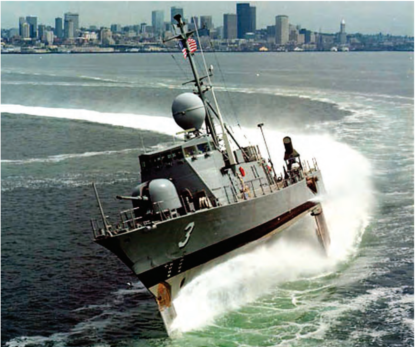
The Boeing Patrol Hydrofoil Missile U.S.S. TAURUS (PHM-3) takes a high-speed turn on her underwater foils during sea trials in 1977, on Elliott Bay, in Seattle. At 132-feet long, this PEGASUS-Class hydrofoil—and her five sister military patrol vessels—were the largest built by the Boeing Marine Systems division. Photo courtesy The Boeing Company.
