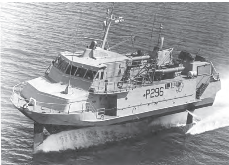
A military variant of the Boeing 929 commercial Jetfoil, HMS SPEEDY, was built for Britain's Royal Navy and went into service in June, 1980. The 90-foot, 50 knot capable hydrofoil was used as a fisheries patrol vessel off the Shetland Islands in the North Sea. Photo courtesy of Hal Turner.
