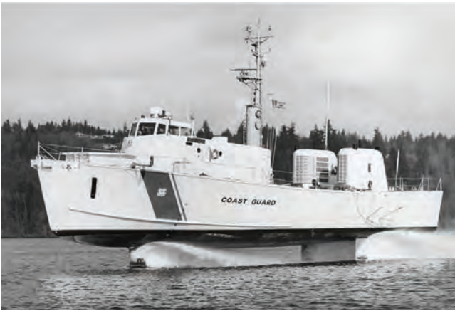
Left: Shown in her U.S. Coast Guard paint scheme in Puget Sound, in 1975, at the beginning of her evaluation by the sea service; the hydrofoil HIGH POINT (PCH-1) was designed by Boeing and built by J.M. Martinac Shipbuilding of Tacoma. This 116-foot hydrofoil, capable of speeds of more than 50 knots, was built under Navy contract, placed in service in 1963, and was the company's first military hydrofoil. Photo courtesy Coast Guard Museum Northwest.
