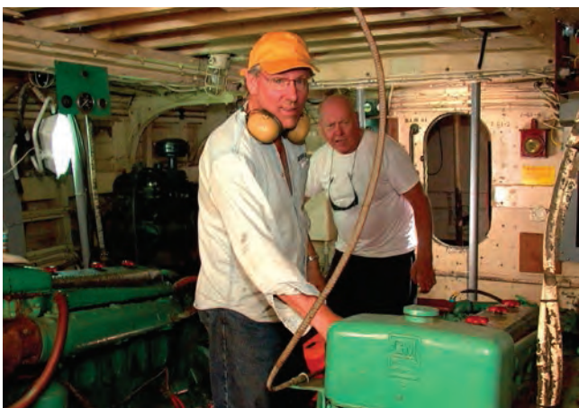
Left: Dan and his Air Force veteran friend Royal Journey are seen doing maintenance on one of CG-83527's twin General Motors 671 diesel engines. Originally powered by two 600-horsepower Sterling Viking gas engines, almost all of the cutters were re-equipped with less fuel-hungry diesels after they were decommissioned and sold in the commercial market. Photo by Marc Bracken.
