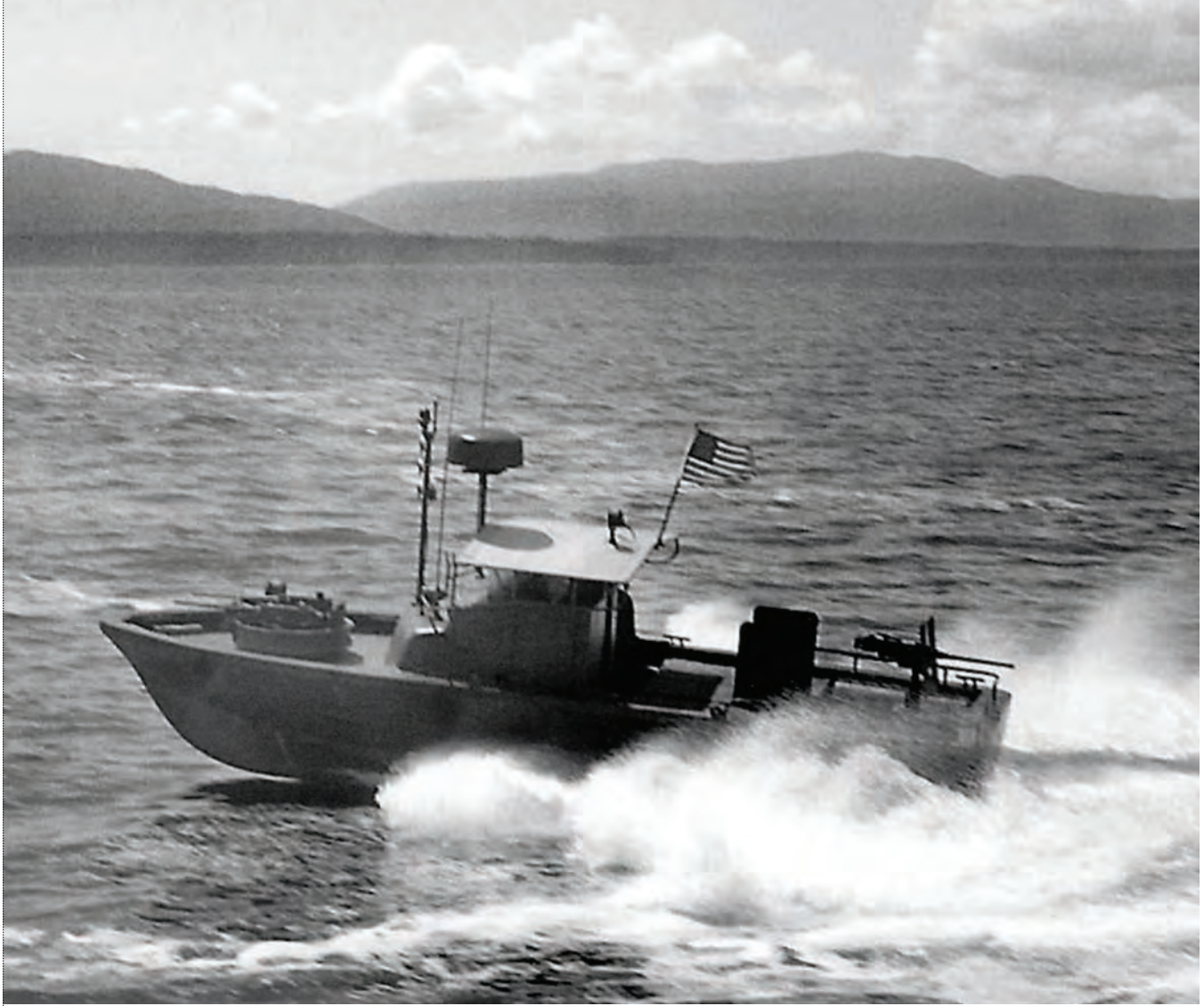
A United Boat Builders 31-foot Navy PBR (Patrol Boat River) completes a 180 degree, hairpin turn on Bellingham Bay during sea trials in 1966. The company built about 250 of the fast, maneuverable patrol boats for the Navy and Army during the Vietnam War. Photo courtesy Don Rubeneck.
