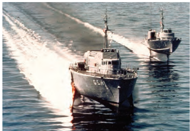
U.S.S. PLAINVIEW (AGEH-1), (left) and HIGH POINT (PGH-1) are shown flying above Puget Sound on their foils during evaluation runs in July, 1978. The 220-foot PLAINVIEW, the Navy's largest hydrofoil, was built by Lockheed Shipbuilding and Construction Company of Seattle, and commissioned in March, 1969. Photo courtesy of Navy History and Heritage Command, Photographic Section.
