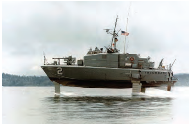
Left: Shown in her U.S. Coast Guard paint scheme in Puget Sound, in 1975, at the beginning of her evaluation by the sea service; the hydrofoil HIGH POINT (PCH-1) was designed by Boeing and built by J.M. Martinac Shipbuilding of Tacoma. This 116-foot hydrofoil, capable of speeds of more than 50 knots, was built under Navy contract, placed in service in 1963, and was the company's first military hydrofoil. Photo courtesy Coast Guard Museum Northwest.
