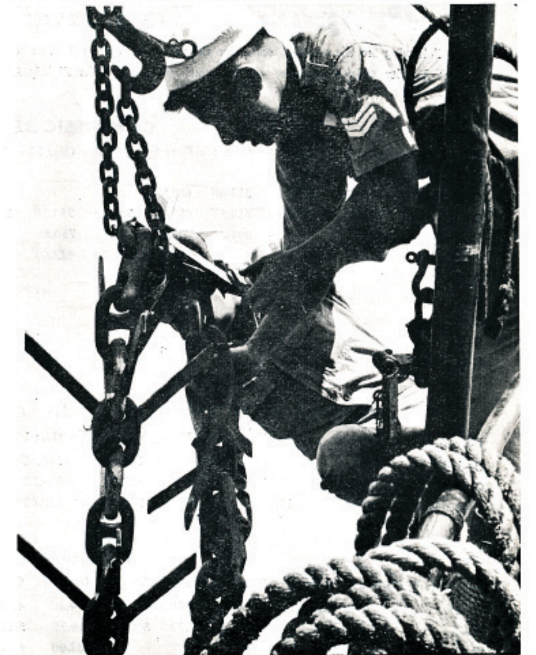
CUTTER STUDS — Vietnamese Navy sailors inspect the cutter studs on the chain-drag minesweeping gear aboard a Vietnamese LCMM prior to the morning sweep of the Dong Nai River. (Official U.S. Navy Photograph by LTJG J.F. Pfaff)
