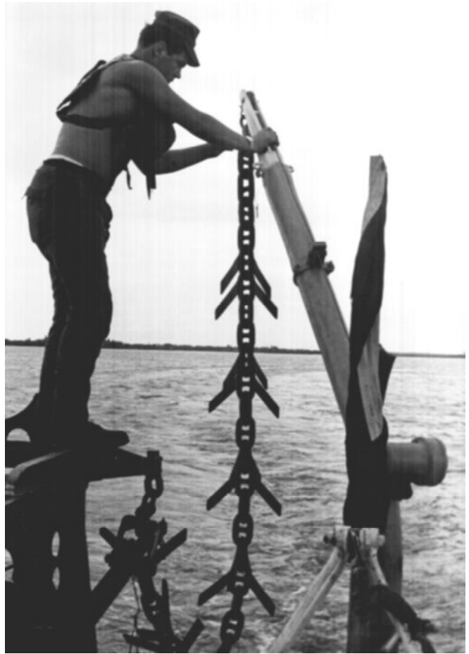
Deploying Chain-Drag Sweep
